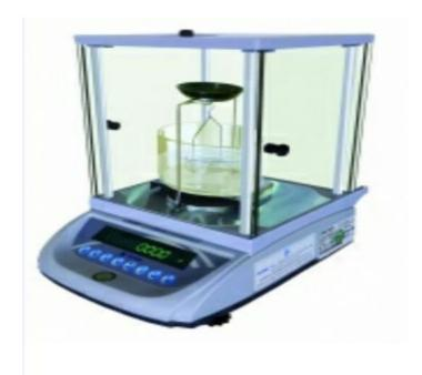
This is basic Requirment of all Polymer Industry to find out Material Density. which effect most of Its Parameters and Quality of products. Such as Mixing with Other agent, Flow, shining, straingth, Tensile and Modulus Properties etc.
