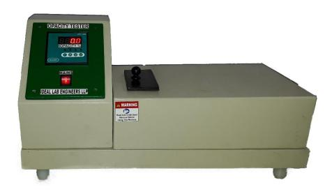
IDEAL LAB ENGINEERS Opacity Tester ,used to determine optical characteristics of plastics films/pipe/paper. Procedure based on transmission of light through the specimen.
