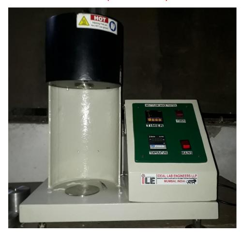
The Melt Flow Index Tester measures the rate of extrusion of a Thermoplastic Material through orifice of Specific Length and Diameter under prescribed conditions of temperature and pressure.
