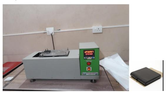
A packaging film's "coefficient of friction" (COF) provides a relative indication of frictional characteristics. Controlling COF gives processors the ability to optimize performance and avoid problems in forming, transporting, and storing of packages.
