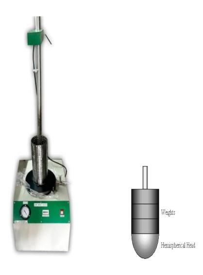
The Dart Drop Test, also referred to as Falling Dart Impact Test or Free Falling Dart Method, is a conventional method to evaluate the impact strength or the toughness of a polymer film. A dart with a variable weight falls from a defined height on a crease-free and fixed film.
