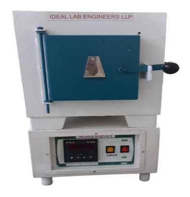
ASH CONTENT TESTER/FILLER TESTER: This is basic Requirment of all polymer industry to find out percentage % of Impurities/ filler mixed in polymer this parameter directly effect the Quality of Polymer and its products.
