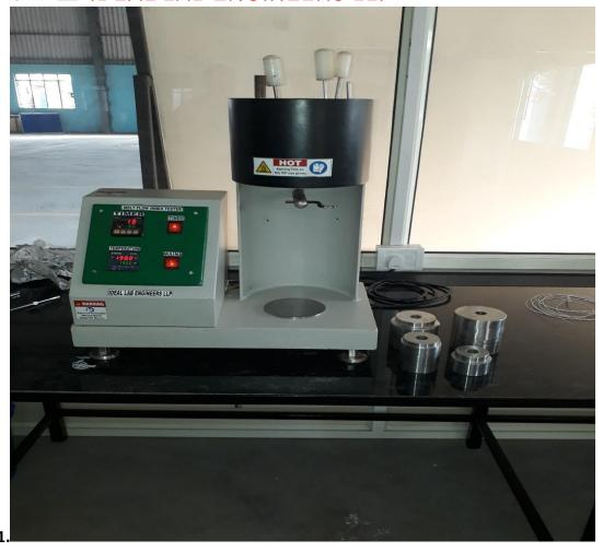
The Melt Flow Index Tester measures the rate of extrusion of a Thermoplastic Material through orifice of Specific Length and Diameter under prescribed conditions of temperature and pressure.
